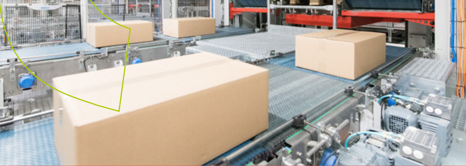
TGW Logistics efficient „FullPick“ solution for fully automated picking of mixed pallets
